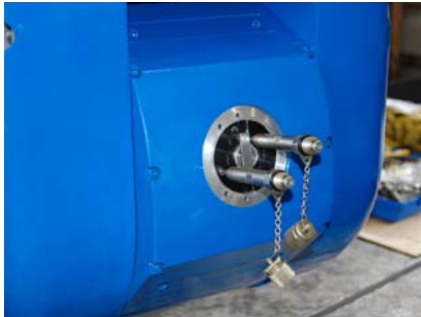
Swivelled A-axis with stems and fittings on bleeding points
