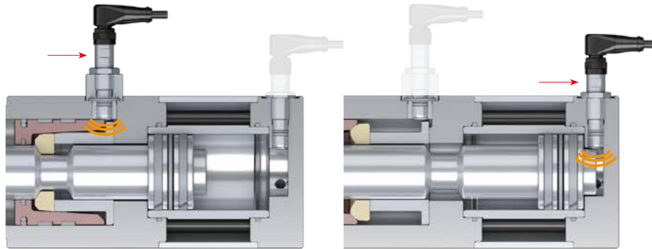
Inductive sensor: inquiry of locking and extended position of the piston rod (order code SL...)
