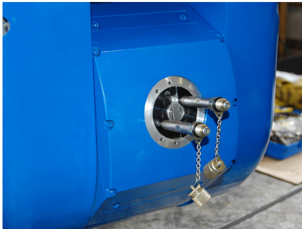
Stems and fittings on bleeding points
