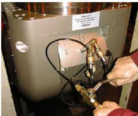
Bleeding set with closed blocking tap, attached to the ports of the clamp and release line on the swivel housing of the milling head.
