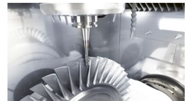
Dynamic positioning: Machining of aircraft turbine element
