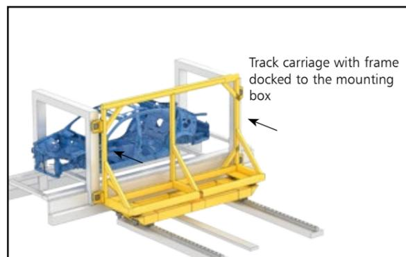
The clamping frame is locked to the carriage very precisely and with high rigidity. The repeatability lies in one hundredth millimeter range.
