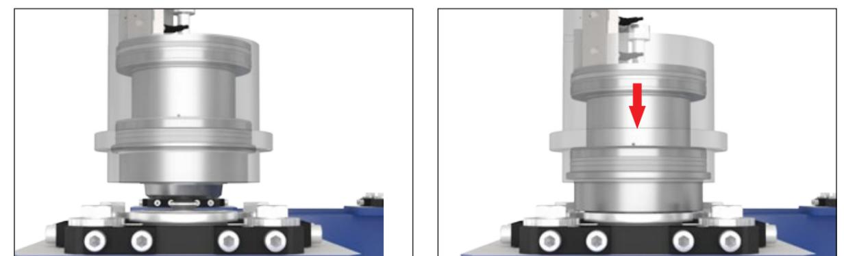
Transfer of hanging frames with CyTab-Scope: in case of reduced ceiling height the transfer can be executed without Z stroke. The frame is fed in Y(X) direction. There is a gap between frame and clamping unit which enables an even lining. Then the unit moves out and clamps the frame sided flange. With that the same accuracy is achieved that is guaranteed by the standard CyTab unit.
