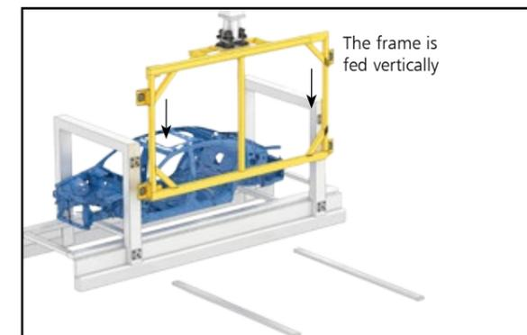
Here also the complete function "gripping • centering • locking" takes place automatically in a single reproducible process. Because of the positive locking the interface is mechanically very stable.
