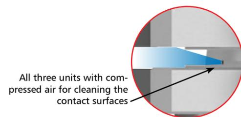
All three units with compressed air for cleaning the contact surfaces
