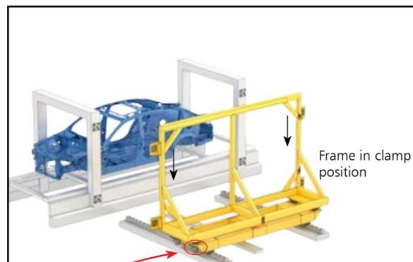
In the following clamping process, the clamping unit is pressurized and grips the flange-bolt with its collet chuck. The complete function "gripping • centering • locking" takes place automatically in a single reproducible process. Because of the positive locking the interface is mechanically very stable.
